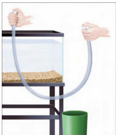
Fill the siphon tube with water and use your thumbs to block both ends.
