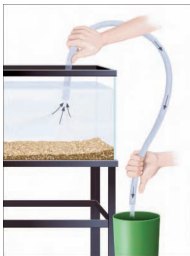
Put one end of the tube in the aquarium and the other end in the bucket. Release your thumbs and water will flow from the tank.
